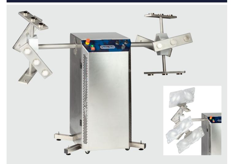
Spinning machines are used to evenly distribute the chocolate in the moulds and to prevent the formation of air bubbles in the chocolate.
